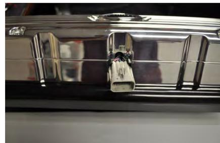
Apply Anti-Seize to the threads of the 1/4-20 X 1-1/4 ARP 12pt. cap screws. Install top billet coil cover carefully not to pinch coil harness and tighten.
