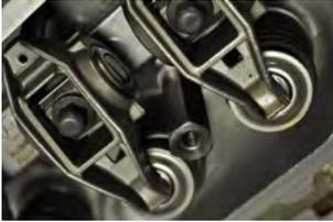
Install spacer nuts into cylinder head and torque to 45 inch-pounds.
